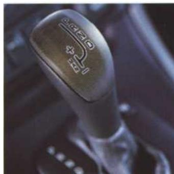
The four-speed Geartronic automatic transmission can also be shifted manually, if you want a more active driving style. You can shift up by pushing the lever away from you and down by pulling it towards you (Volvo S80 T6 SE only).
